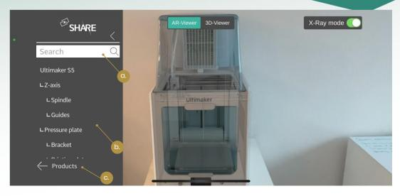
Figure 88: 3D model of the printer superimposed over the physical printer (a. Search for (sub)components; b. Product tree; c. Back to product list)
