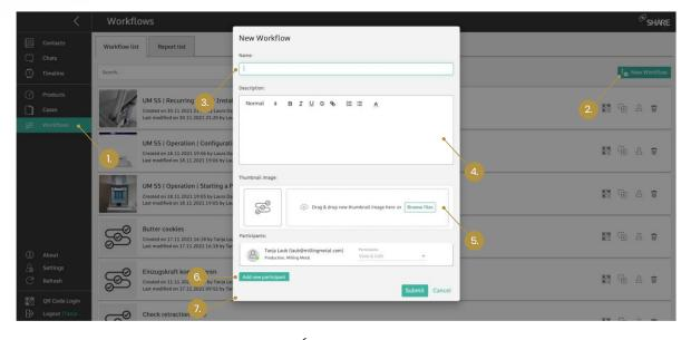
Figure 93: Creating a new workflow (1. Open Workflows module; 2. Select 'New Workflow'; 3. Enter a name; 4. Enter a description; 5. Add a thumbnail image; 6. Add participants and assign permissions; 7. Scroll down to add products to the workflow)
